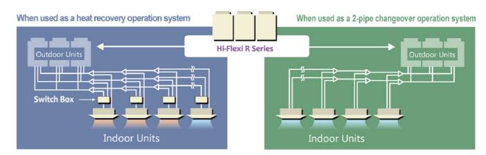
Common outdoor units are applicable to the heat recovery operation system as well as the 2-pipe changeover operation system. This eases the burden of review work when designing the equipment layout, while reducing the workload of installation on site.
