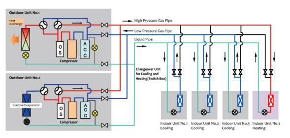
When total indoor heating load is less than cooling load, heat is being transferred from cooling room to heating room, part of heat exchanger is used as condenser to exhaust the redundant heat.
