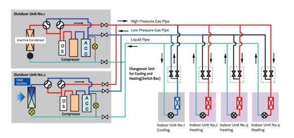
When total indoor heating load is more than cooling load, heat is being transferred from cooling room to heating room, part of heat exchanger is used as evaporator to compensate the required heat.
