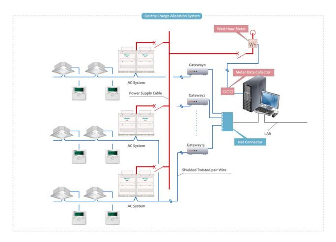
All the indoor units and outdoor units connected with one adapter comprise one communication BUS system . Max.64 outdoor units and 160 indoor units can be connected to a BUS system. Max.16 adapters can be controlled by one computer.
