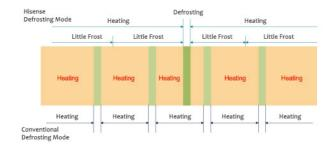
Outdoor unit adopts the outdoor temperature sensor and heat exchanger temperature sensor, and precisely calculates the defrosting time.
